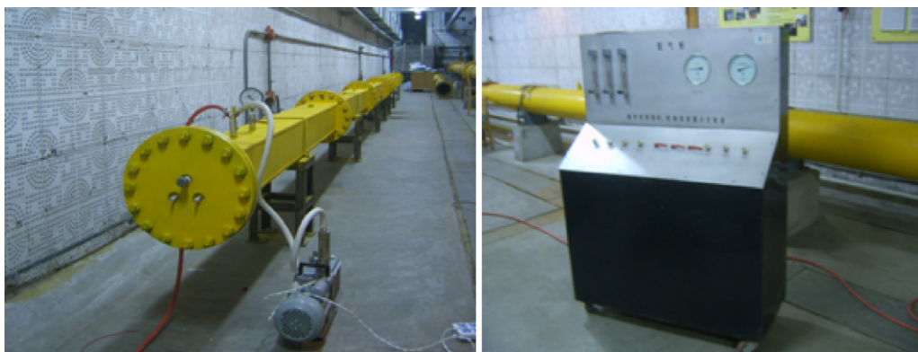
Fig. 2. Gas explosion pipe and gas mixing system.
